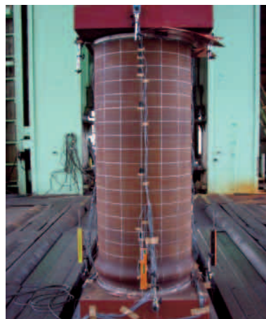
Photo 3 Shell wrinkle after a compression test
